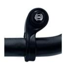
Pressing the RBS button will activate this function which allows the engine to slow down in descent and charge the battery at the same time.
