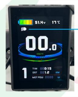
\*To turn the headlight on/off, press and hold the UP button for 3 seconds
