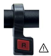
When reverse gear is engaged (pressing the button once), the display will show REVERSE flashing in orange.
