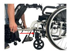
14. If necessary, act on the dowels of the depth regulator to adjust the distance of the handlebar from the user, moving the regulator closer or further away along the arm, then tighten with a tightening torque of 12Nm.
