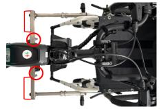
13. Unscrew the side tightening levers and check that both conical pins enter and exit freely from the respective depth regulators, moving the thruster further away and closer. Then tighten the clamp screws with weighting (5-12 Nm), taking care not to damage the wheelchair tubing.
