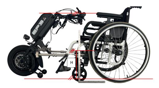
2. Set the wheelchair's parking brakes and place the thruster in front of the wheelchair with the wheel in the center of the wheelchair
