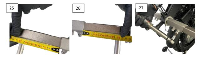
12. If necessary, turn the depth adjuster grub screws to adjust the distance of the handlebar from the user, bringing the adjuster closer to or further away from the user, then tighten to a torque of 12 Nm.
