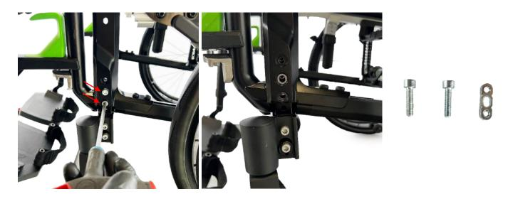
2. Insert the M6x30 screw from the outer side into the centre hole (fig. 4). Insert two washers on the opposite end on the inside (fig. 5), then lightly screw in the M6 flange nut (fig. 6).
